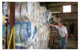
THE PROCESS When breaking down mattresses into components, recyclers bale and count fabrics.
