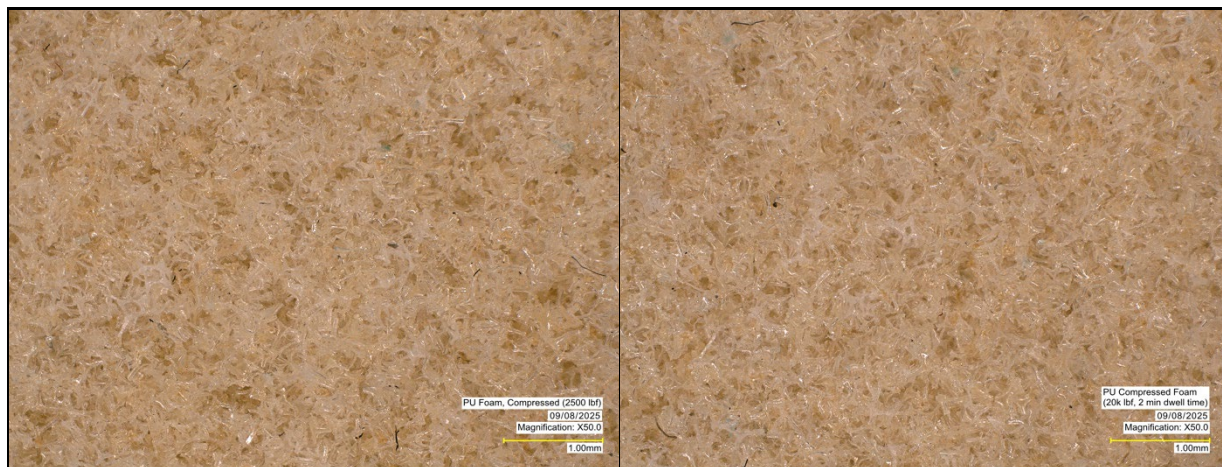
Figure 15: Compressed PU Foam Powder Sheets (50x). Image shows two samples of compressed foam powder: 2500 pounds-force (left) and 20,000 pounds-force (right). While there is interlocking of foam pieces in the sample on the left, there is noticeably more in the sample on the right, which was compressed at a higher compressive force.
