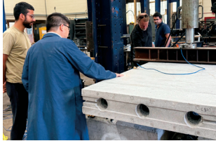
Testing of full-size Panel with Mattress Foam Core
