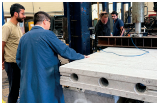
Testing of full-size Panel with Mattress Foam Core
